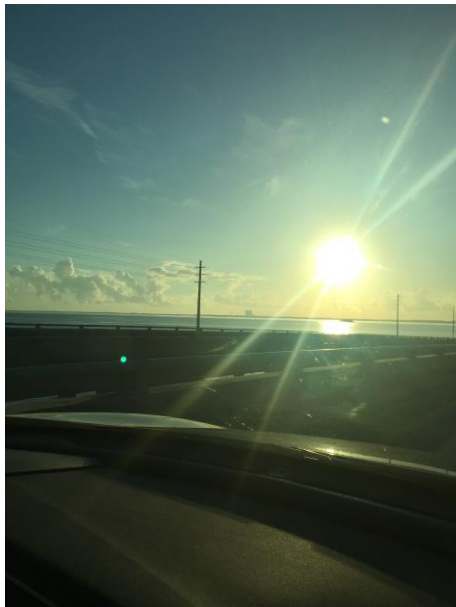
Figure 1. CMOS Sensor Blooming. An example of sensor bloom is seen here. The number of electrons converted from the sun overflow into surrounding pixels, producing the hazy shape of the sun.
